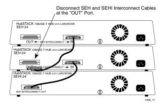
Figure 3-7. Disconnecting the HubSTACK Interconnect Cable
